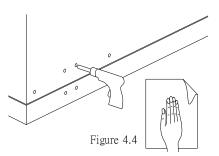
die screwing depth. WTA series linear scale is tightened with M4 screw, and WTB with M5. After drilling holes on the installation surface, you have to smooth the granulated surface and clean the paint and the stains (Figure4.4).
