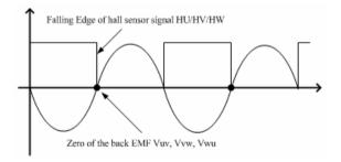
Figure 4-1: Back EMF and hall sensor sequence requirement of the ACS306
