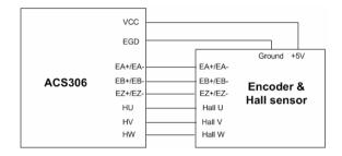
Figure 3-4: The ACS306 supplies the encoder directly
