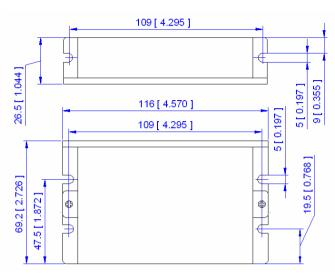
Figure 2-1: Mechanical specifications
