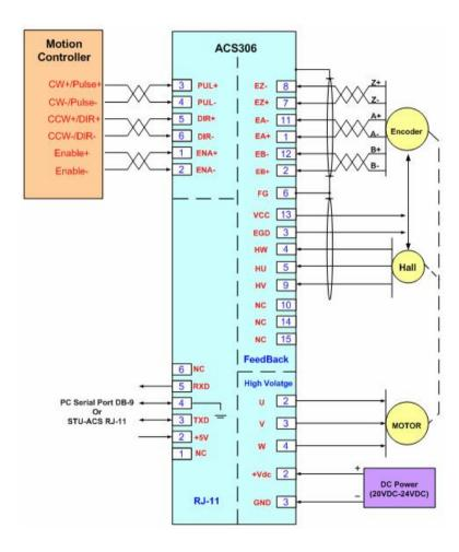
Figure 3-7: Typical connection of the ACS306
