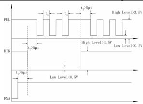
Figure 5-2: Sequence chart of control signals
