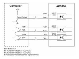
Figure 3-1: Connections to controller with differential outputs
